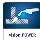
**vision.POWER** for a more concentrated arc and deeper penetration on medium and thick thickness
